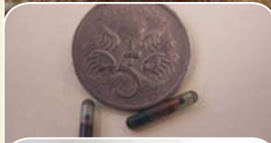
PIT tags used for identifying fish in hatcheries.
