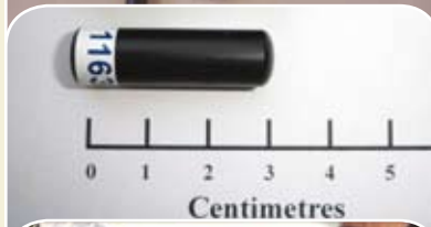
Acoustic tag used for tracking fish movement (photo courtesy of TAFI).
