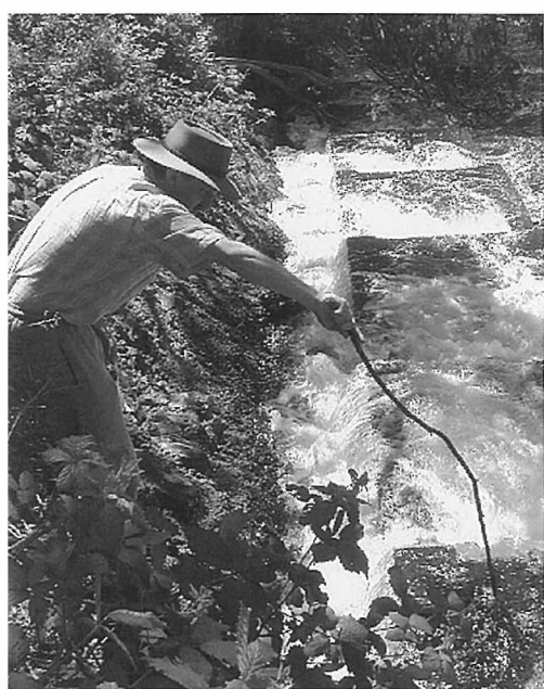
Dr Martin Mallen-Cooper measuring the depth of the pools in the fish ladder on the Emu River.
