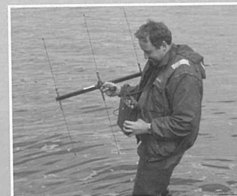
Using a bio-telemetry receiver to locate transmitter carrying carp and hopefully his companions. Photo Dave Jarvis
